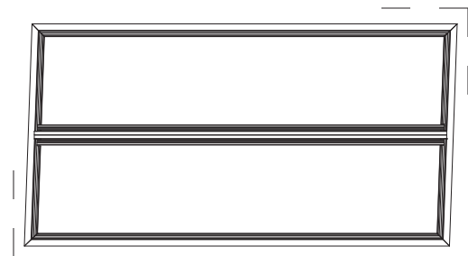
INCORRECT INSTALLATION. FRAME NOT SQUARE
